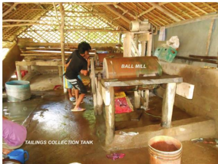
The ball mill facility of the mining operation, where mercury is used to process gold ore One of the sites from where the scientists collected water
